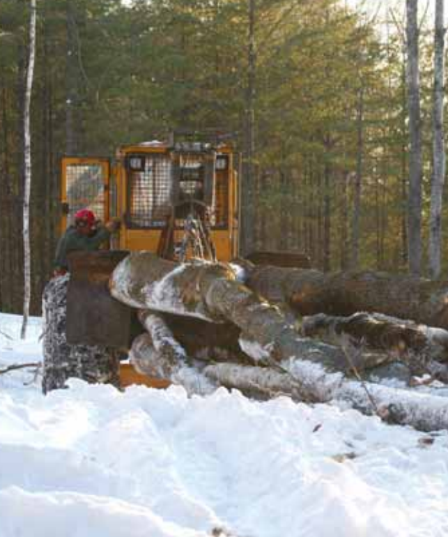
Top: Skidding logs on frozen ground minimizes damage to soils. Bottom: A good logger will take measures to avoid and protect wet areas when skidding logs.
